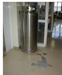
7. **Property Damage: Cryogenics can damage rubber tubing and crack floor tiles if spilled.** Special care should be taken to avoid spilling any cryogenics. Cracked floor tiles may also present a tripping hazard to other workers. Notify your Building Administrator of any floor tiles that require repair.
