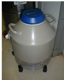
**Dewar:** an insulated container used to store and transport liquefied gases. It is insulated by a vacuum between its two walls and is equipped with pressure relief device(s).
